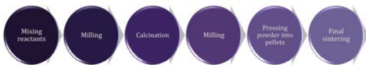
Figure 4.1. Schematic representation of the solid-state reaction route used for the synthesis of the \text{BaCe}_{0.6}\text{Zr}_{0.2}\text{Y}_{0.2-x}\text{M}_x\text{O}_{3-\delta} ( \text{M} = \text{Fe}, \text{Pr}, \text{Tb} ) and \text{SrFe}_{1-x}\text{Co}_x\text{O}_{3-\delta} samples.
