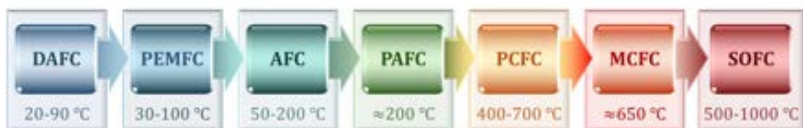
Figure 1.1. Schematic overview of the types of fuel cells with the corresponding typical operation temperatures: direct alcohol fuel cell (DAFC), proton exchange membrane fuel cell (PEMFC), alkaline fuel cell (AFC), phosphoric acid fuel cell (PAFC), protonic ceramic fuel cell (PCFC), molten carbonate fuel cell (MCFC), and solid oxide fuel cell (SOFC) with oxygen-ion conducting electrolytes. The illustration was prepared based on information provided by Samsudin et al. and Zhang et al. 1,2
